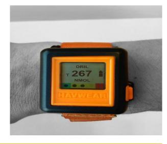
Figure 1 Reactec wearable HAVS monitor
